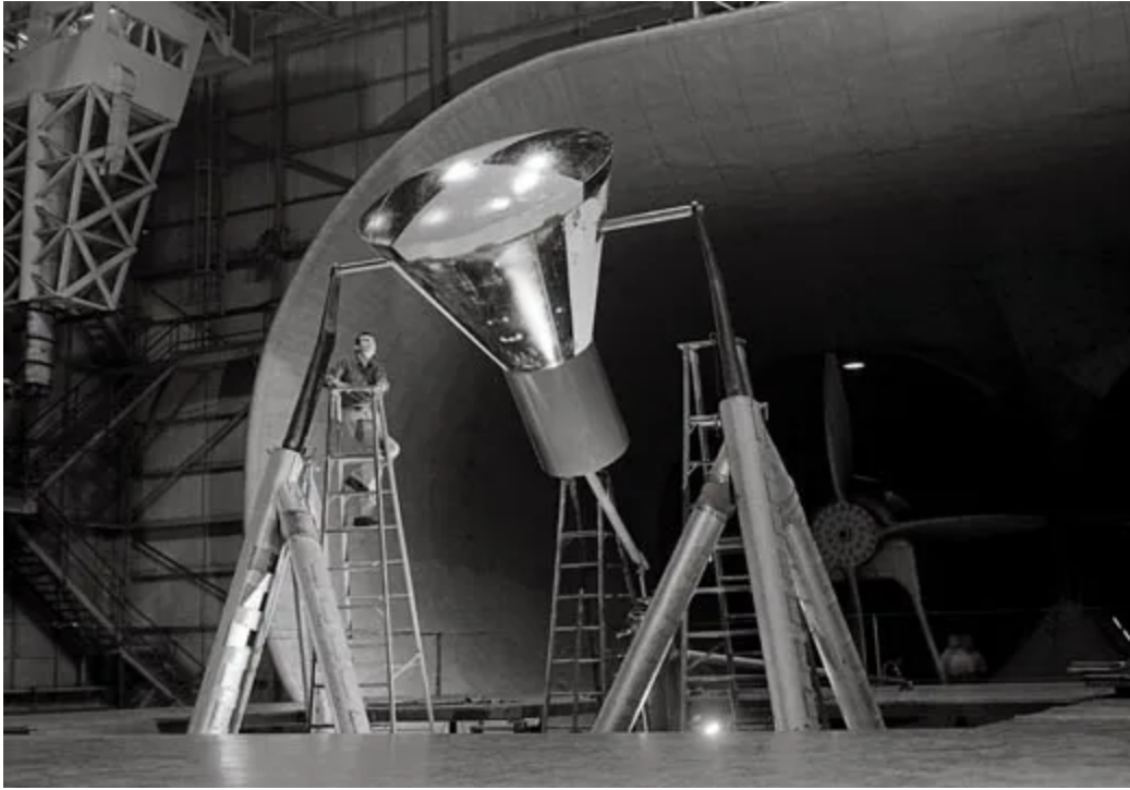
The Mercury space capsule during a 1959 wind tunnel test. NASA Langley Research Center
