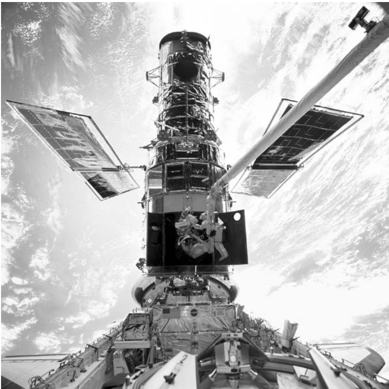
Astronaut John M. Grunsfeld, positioned on a foot restraint on the end of Discovery's remote manipulator system (RMS), prepares to replace a radio transmitter in one of the Hubble Space Telescope's electronics bay. (NASA Image # STS103-713-048)
