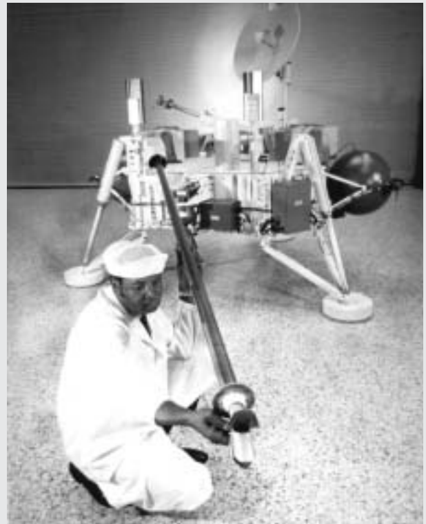
Viking Lander soil sampler arm being tested, 1971.
