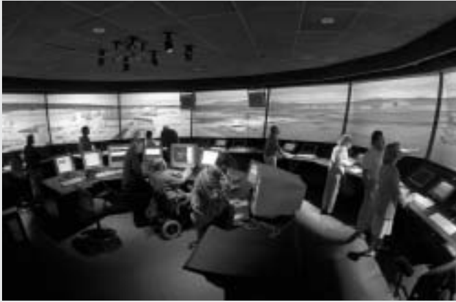
Ames' virtual airport, FutureFlight Central, 1995, is used to study improvements to air traffic control.
