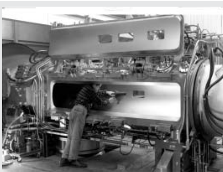
A lifting-body model being installed in Ames' 3.5-foot hypersonic wind tunnel.
