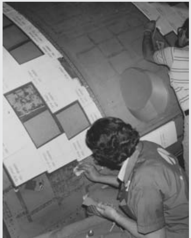
Ceramic tiles being mounted on a shuttle orbiter, 1980.
