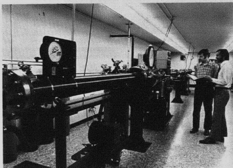
SHOCK TUBE in Stanford's High Temperature Gas Dynamics Laboratory can simulate spacecraft shock waves up to Mach 10, over 7,500 mph. Loaned to the University's Mechanical Engineering Department by Ames Research Center, the device is being used in studies of smog and space shuttle effects by research associate Dr. Ronald K. Hanson (left) and Prof. Charles H. Kruger.
