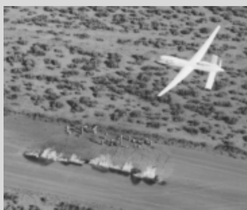
The Altus II remotely piloted experimental 'uninhabited aerial vehicle' (UAV) flying over the test fire at El Mirage, Calif.
