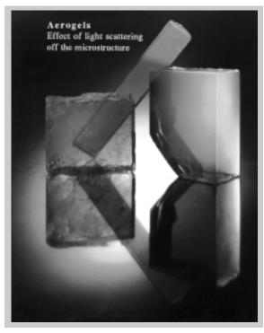
A new concept for spacecraft tiles can be used on Earth to make efficient, vacuum-like insulation for refrigerators, furnaces and automobile catalytic converters.
