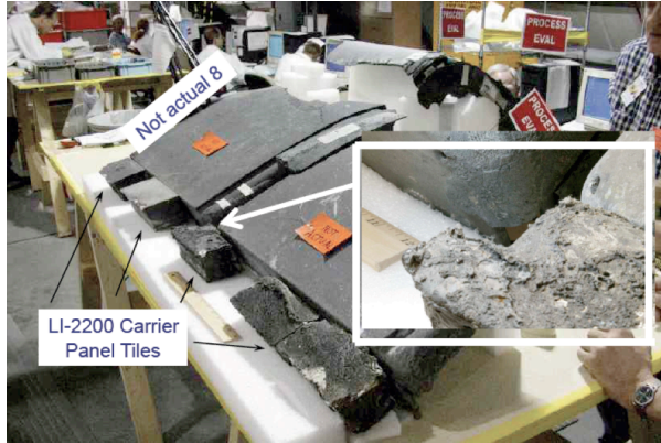
Fig. 8. Photograph of Shuttle Columbia debris that helped pinpoint the location of the foam strike.
