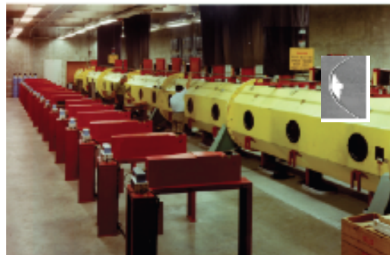
Fig. 10. Photograph of the NASA Ames Ballistic Range showing the test section. The light gas gun launched the model into a counter-flowing supersonic air stream created by a shock tunnel. The black and white inset depicts a shadowgraph of a model in hypersonic flight.
