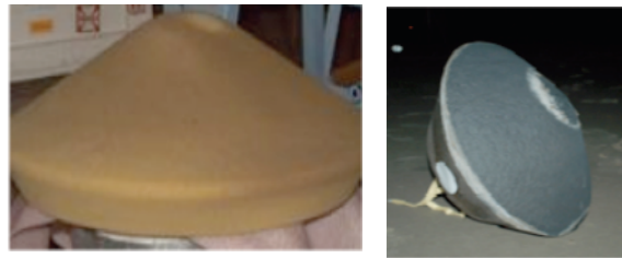
Fig. 5. The Stardust PICA heat shield before (left), and after its return to Earth in January 2006 (right).
