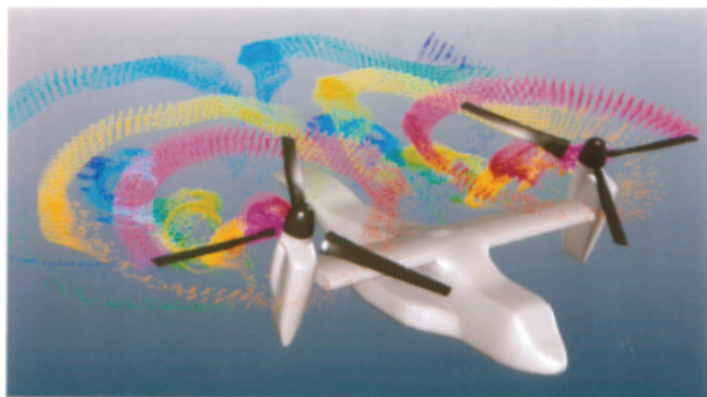
Figure 5. CFD simulation of the V-22 Osprey tiltrotor aircraft at 75 knots [22]. Unsteady particle path traces of the tip vortices.
