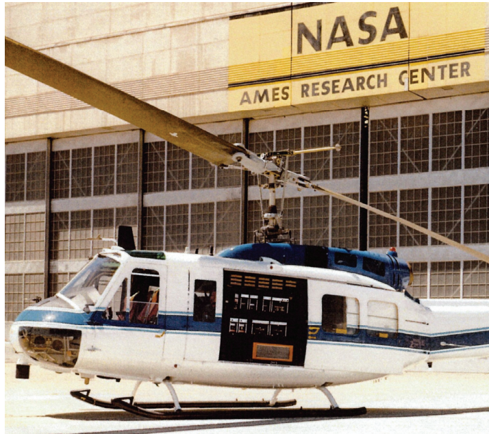
Air-cooled rack of V/STOLAND equipment.
