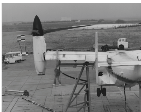
Flow visualization smoke test illustrating the chordwise flow near the wing tip.
