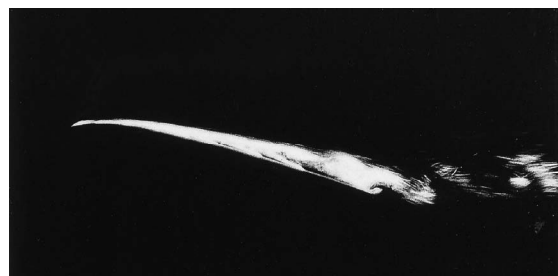
Hydrogen bubbles from surface electrodes.
