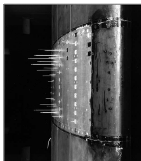
Hot wire “porcupine” array on airfoil surface.
