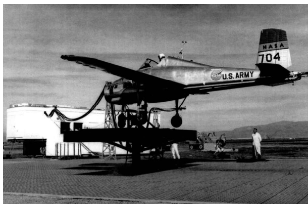
X-14B on tethered test stand.
