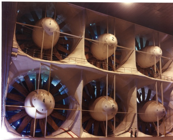
The NFAC drive: six 40-foot-diameter fans with 15 rotor blades and 23 stators per fan.
