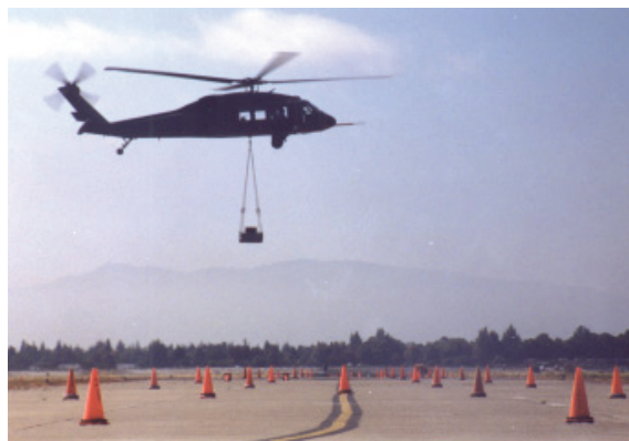
UH-60A with external slung load performing ADS-33 lateral reposition maneuver.
