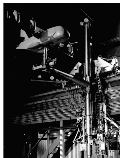
The XC-142 tiltwing VTOL aircraft model mounted on the Princeton University Long Track.
