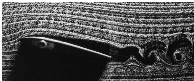
Hydrogen bubbles from a free-stream electrode.
