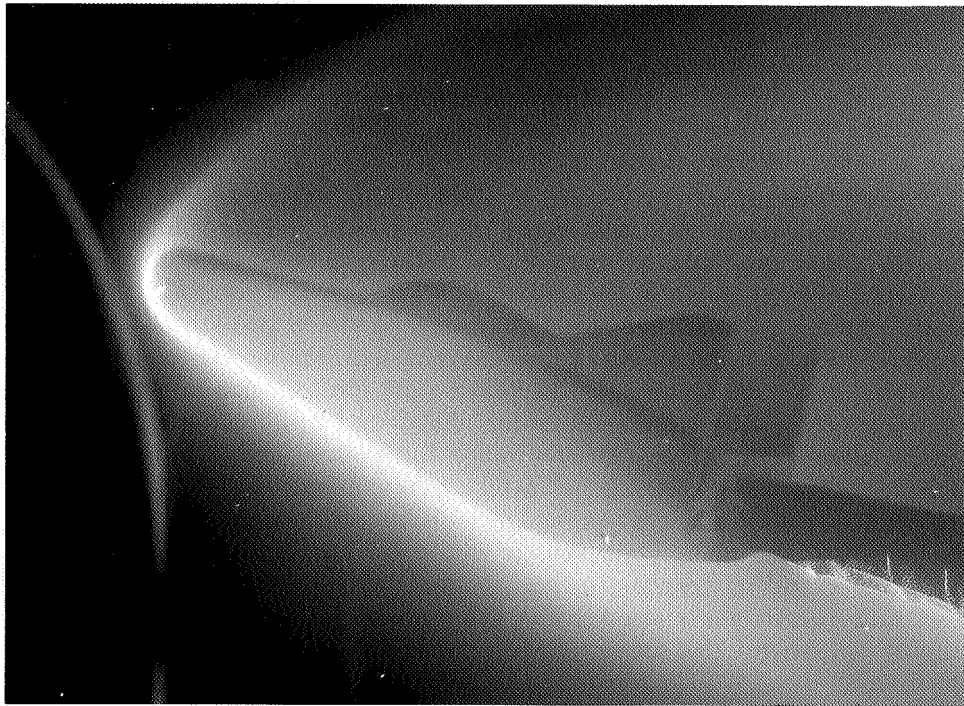
1962. Model of an M-2 lifting body being tested in the Ames Atmospheric Entry Simulator. Obviously, reentry heating would be a problem for the M-2; the tests illustrated the areas of most intense heat and the airflow patterns around the lifting body.
