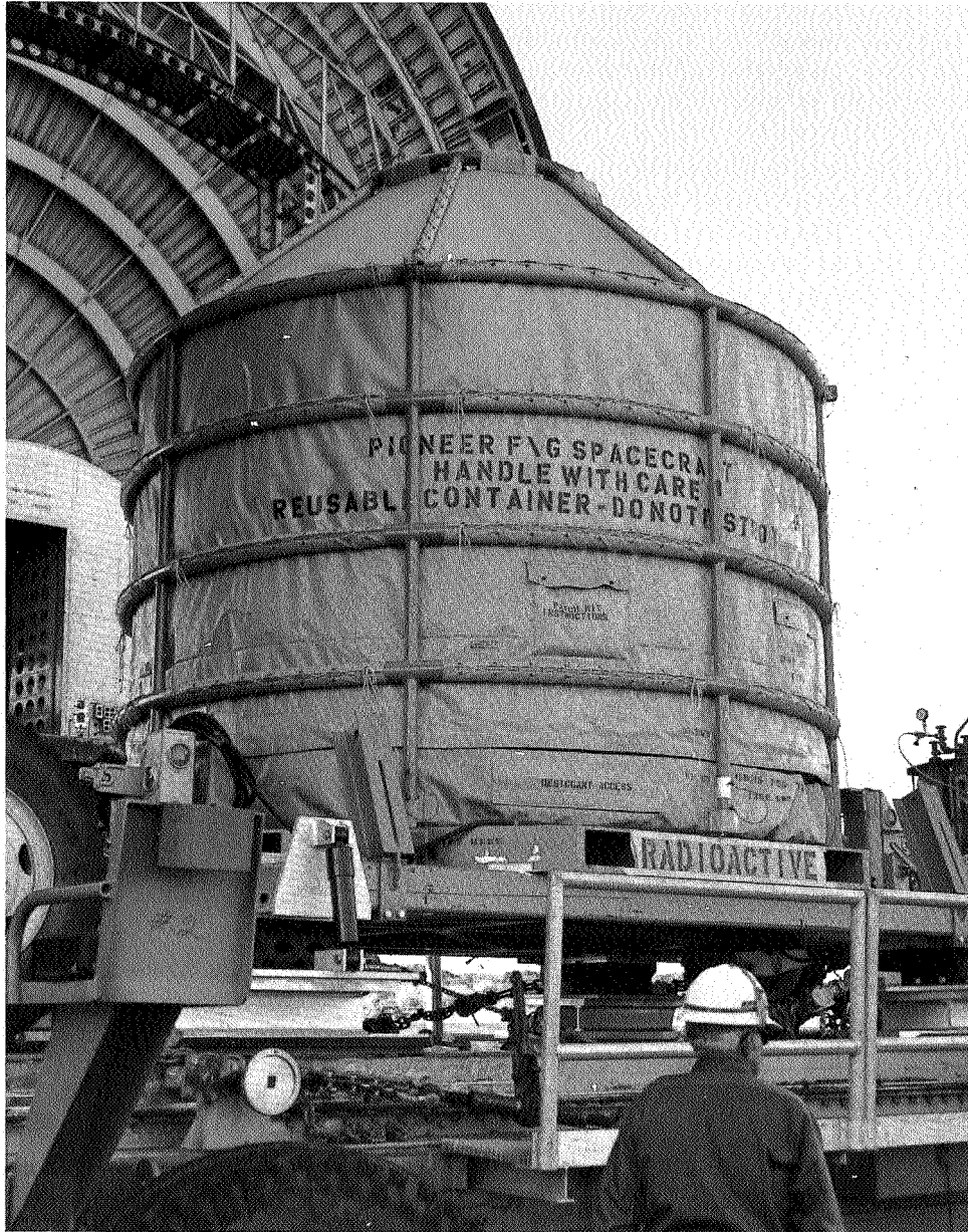
May 1973. Pioneer 17 being unloaded at Cape Kennedy (now Cape Canaveral) prior to launch. (Pioneer 10 had been launched in March 1972.) Note the relatively small size of the Pioneer spacecraft and the reusable packaging protecting it, both typical of Pioneer's thrifty budgeting.
