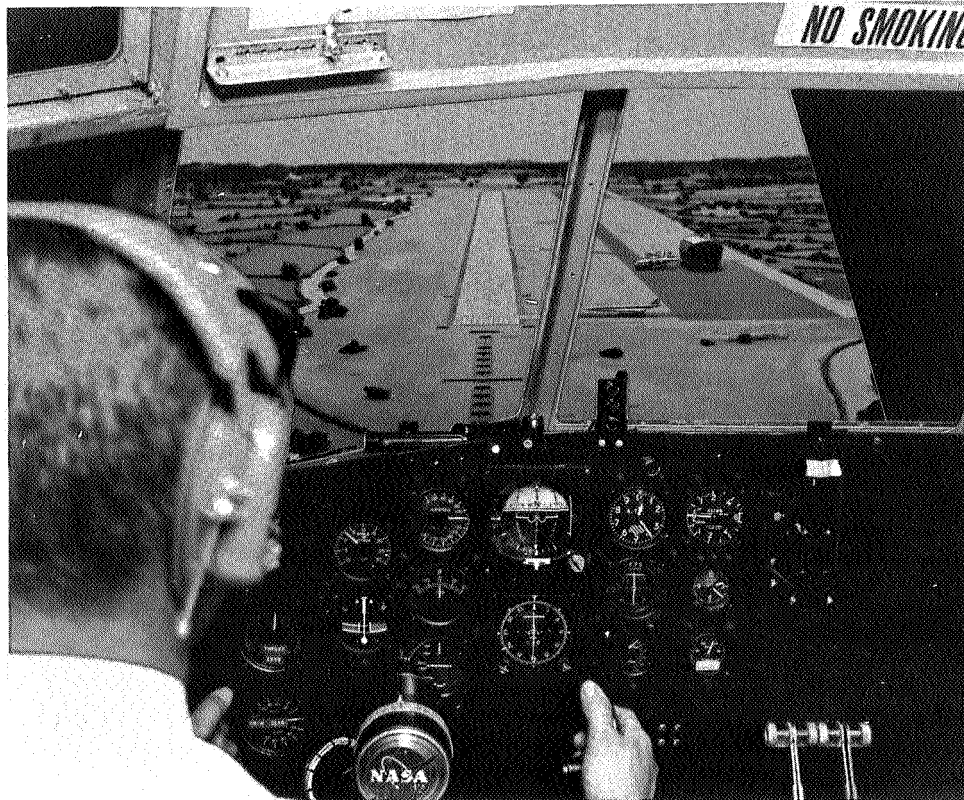
1965. Practicing landing approaches “flying” a double-delta-wing SST in a flight simulator. Such studies test the flight characteristics of aircraft still in the design stage and also monitor pilot performance while making landings.
