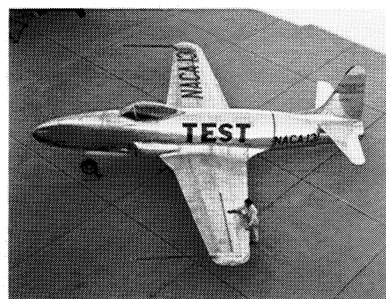
Figure 22 P-80A-1 showing vortex generator installation.
