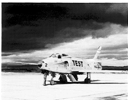
Figure 25 North American YF-93A with NACA submerged inlet.
