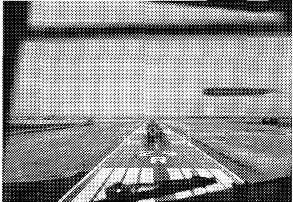
Figure 74 Head-up display mounted in the FAA Boeing 727.
