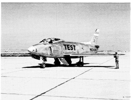
Figure 26 North American YF-93A with scoop inlet.
