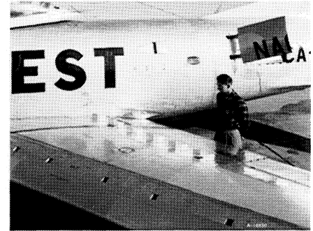
Figure 27 North American YF-86D showing vortex generator installation.
